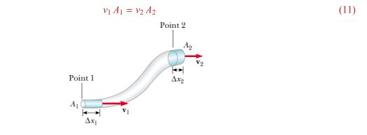
The *Flow* tab in this PHeT Simulation demonstrates the relation between the speed and cross sectional area of an arbitrary pipe.
