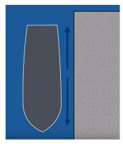
This motion would cause the pressure of the water between the boat and the pier to drop, and the difference in pressure between the water to the left of the boat and to the right of the boat would cause a rightwards force on the boat that would slam it into the pier.
