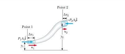
In time  $\Delta t$ , this fluid will flow so that the segment spanning  $\Delta x_1$  across the left cylinder will now span  $\Delta x_2$  across the right cylinder.
